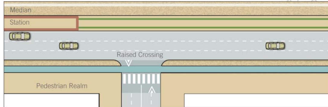
Cycle Track through Minor Junction
