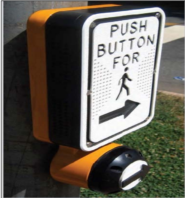
Figure 9. High contrast raised tactile arrow on pushbutton and high-contrast recessed tactile arrow on sign above call button [44].
