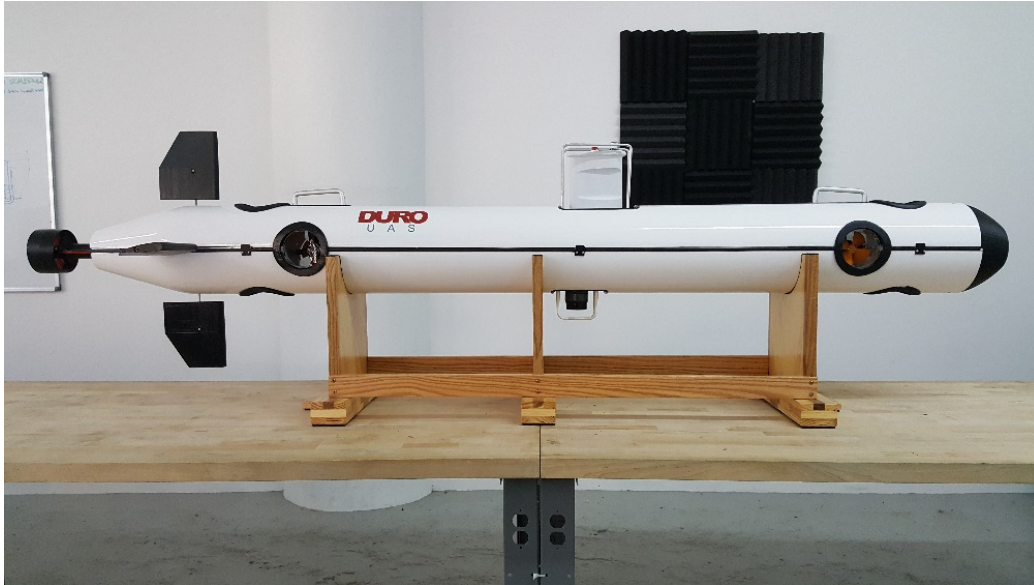
Figure 1. Side view of the Harbor AUV under development for scour monitoring of bridge piers.
