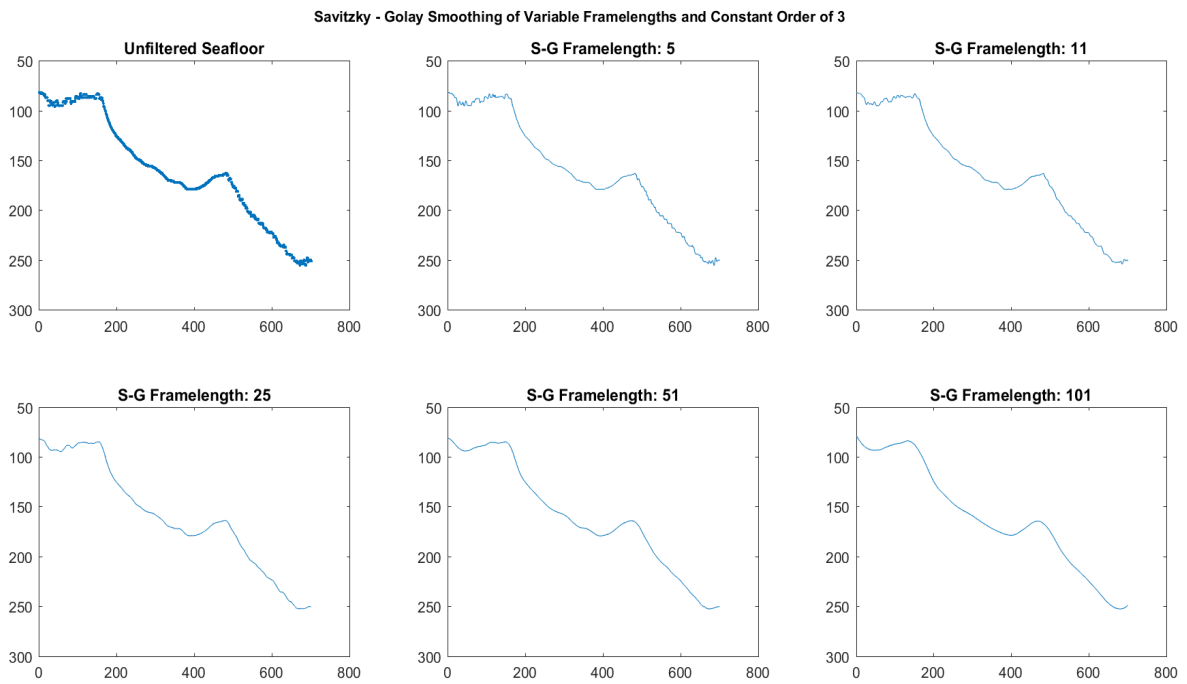
Figure 17. Savitzky-Golay filter at constant frame length and variable orders applied to case 1.
