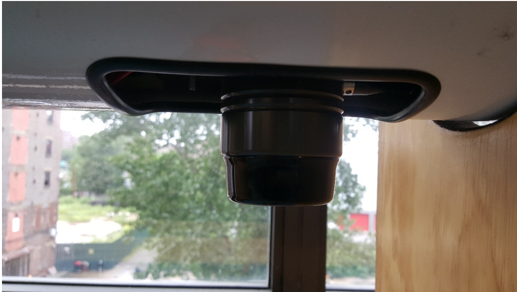
Figure 5. The AUV payload bay, showing the mounted end of the Echologer MRS900.
