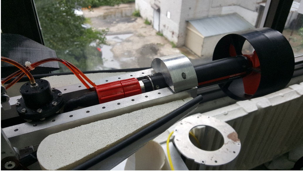
Figure 3. Main rear thruster used in the Harbor AUV.
