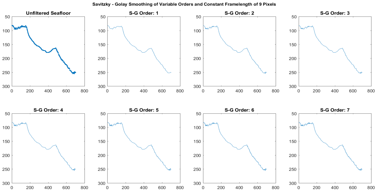
Figure 17. Savitzky-Golay filter at constant frame length and variable orders applied to case 1.
