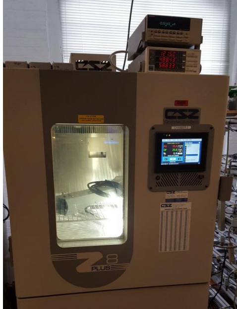
Figure 4. Thermal chamber used to measure performance at different temperatures.
