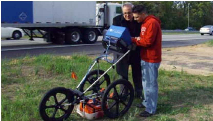
Testing a Ground Penetrating Radar (GPR) Unit for the Location of Fiber Optic Conduits NJDOT/UTRC Project (Fadi Karaa, Associate Professor of Critical Infrastructure, NJIT)
