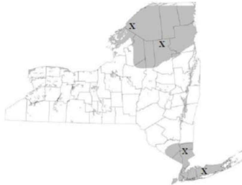
Areas where seasonal models are out of range (in grey) due to the combined effects of median subgrade P.I. greater than 12 and average frost penetration out of range. Possible locations for test sites for this project are marked by X.
